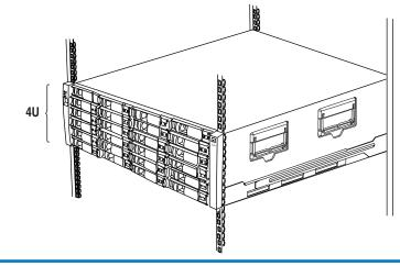
Note: If you are installing the disk shelf in a two-post mid-mount installation, you must use the mid-mount telco kit, which includes brackets, in addition to the two-post telco tray kit.
