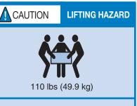
To reduce the weight of the disk shelf, remove the power supplies and IOMs before lifting.
