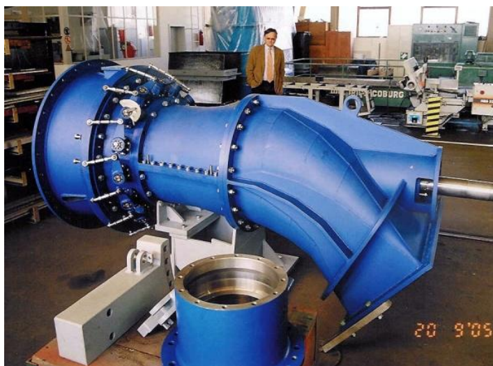
Figure 3 - Example of a Kaplan turbine 9
