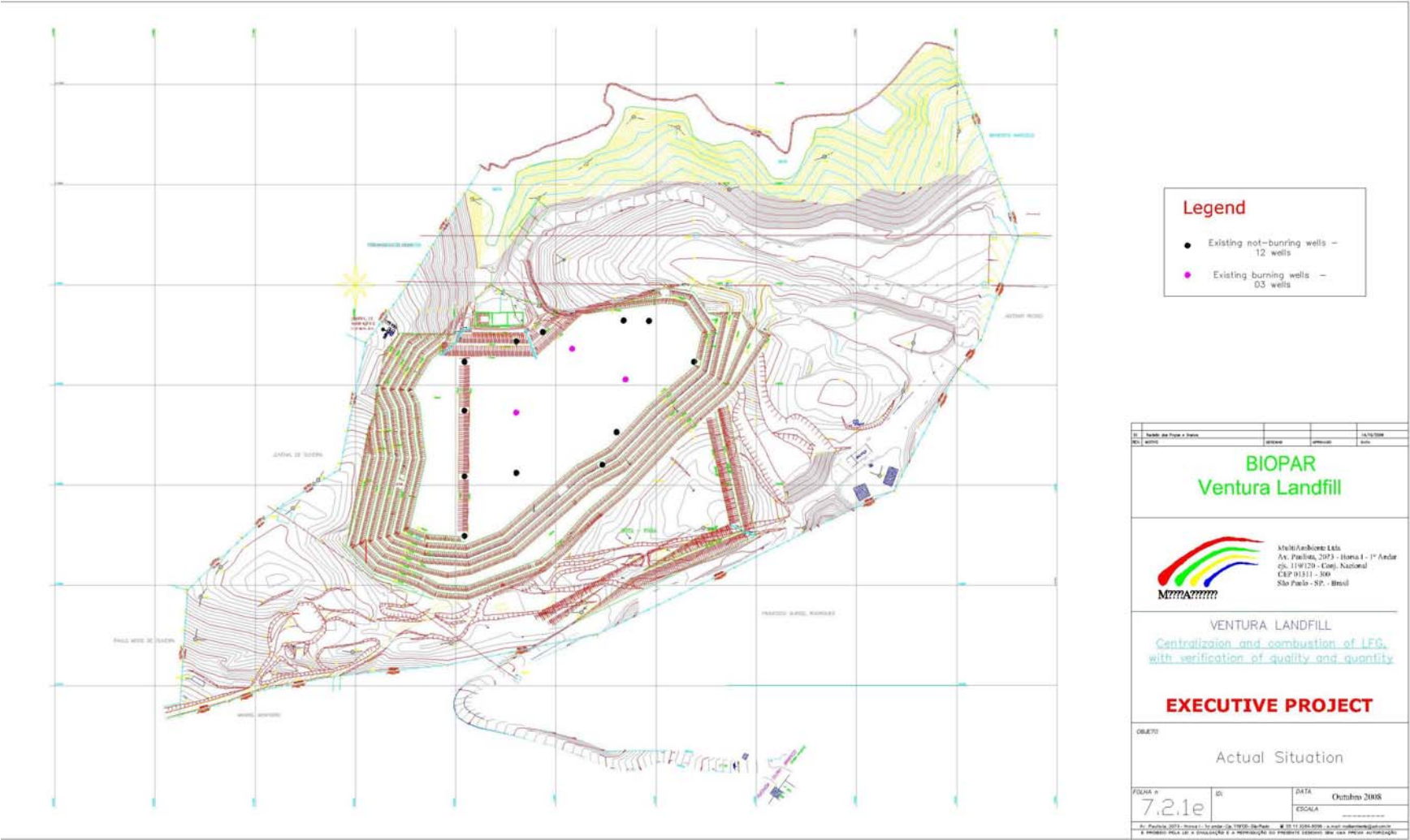
Figure 6. Lay-out of the wells at Ventura Landfill
