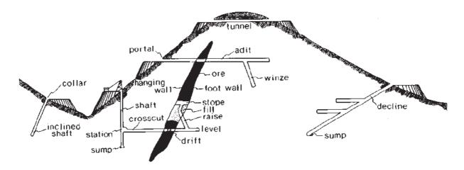
**Development** in an underground mine refers the creation of tunnels and other access routes that will allow the miner to access the ore. Development ends include areas such as:
