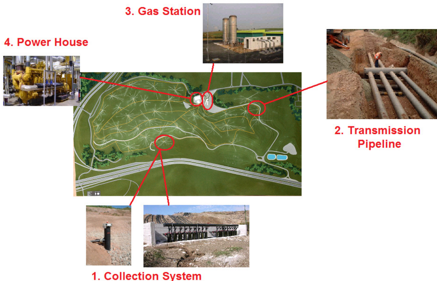
Figure 2. Schematic situation of a landfill with active gas recovery
