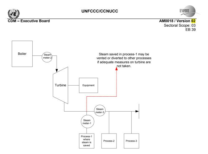
Figure 2: Illustration showing the configuration of a process supplied by back-pressure or extraction steam of a turbine
