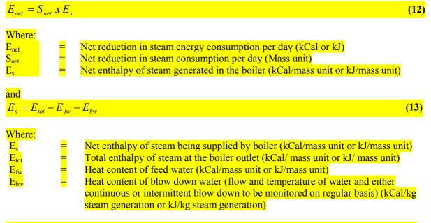
Case-2: Steam supplied is the extraction or backpressure steam of a mechanical steam turbine driving process equipment or a steam turbine producing electricity
