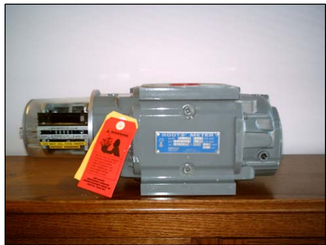
Figure 2. Roots biogas flowmeter
