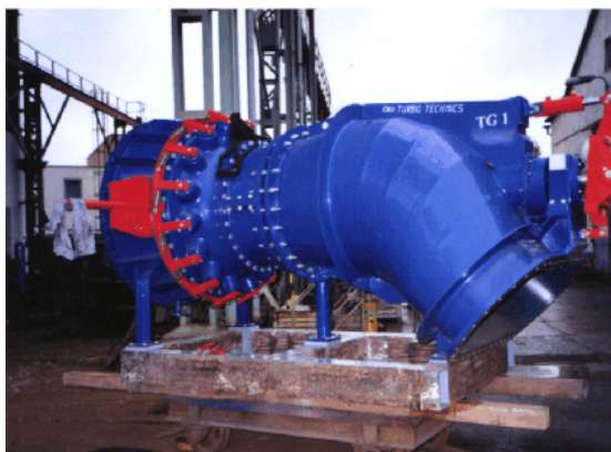
Figure 2 – Example of a Kaplan S Turbine
