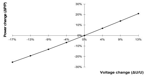
The curve above is not plotted between power and voltage but I presume between percentage difference from 230 V v/s percentage change in power rating.
