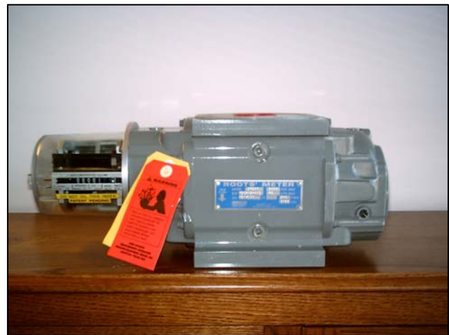
Figure 2. Roots biogas flowmeter
