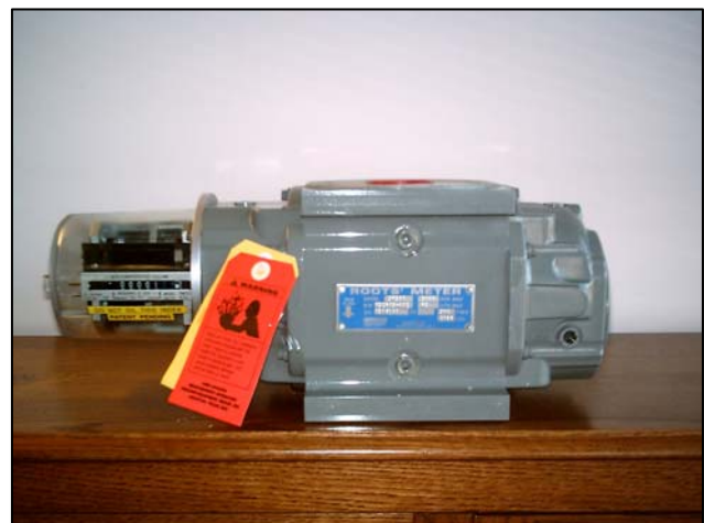
Figure 2. Roots biogas flowmeter
