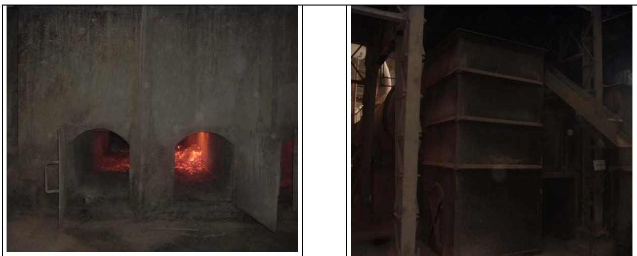
Figure 1: Guará fixed grating furnaces that burn renewable biomass
