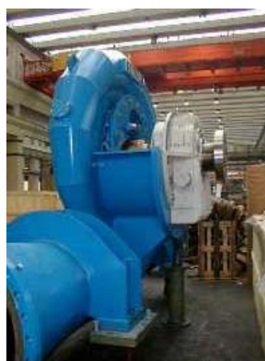
Figure 6 – Francis turbine (Sources: Alstom, http://www.alstom.com.br/ and Water Wheel Factory http://www.waterwheelfactory.com/ ).
