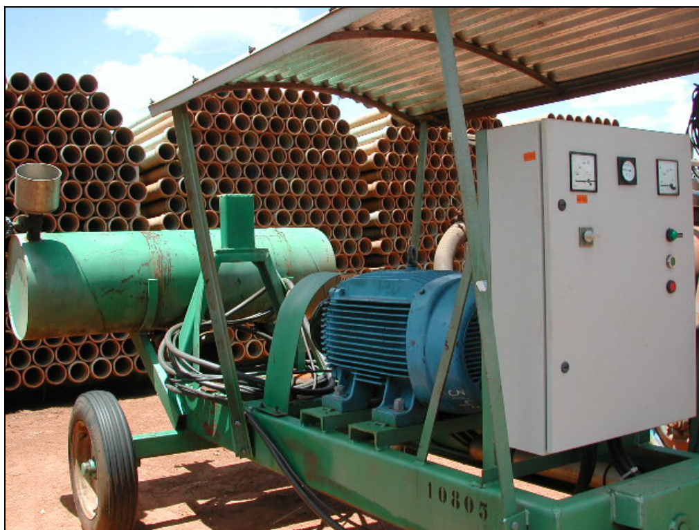
Figure 15: Electric Pumping Station and Control Panel
