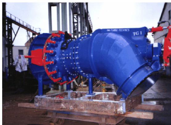
Figure 2 - Example of a Kaplan S Turbine
