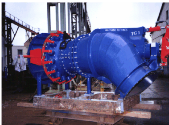
Figure 2 - Example of a Kaplan S Turbine
