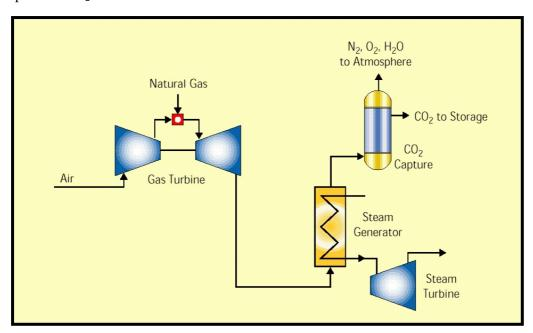
Figure 1. Gas turbine combined cycle with post-combustion capture of CO<sub>2</sub> (courtesy of the IEA Greenhouse Gas R&D Programme).
