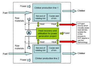
Figure 1. Schematic of sample Project Activity
